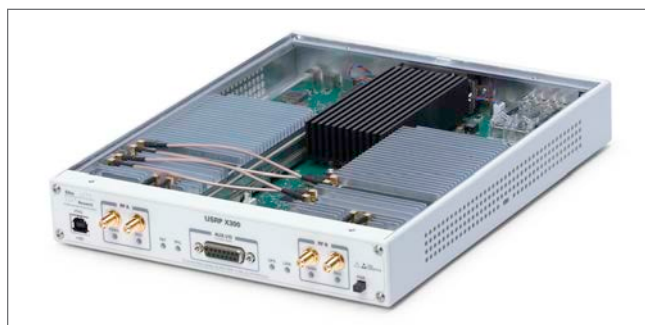
Figure 2 | Two super-heterodyne TwinRX daughtercards inside an Ettus USRP X310 SDR for four phase-aligned RX channels.
