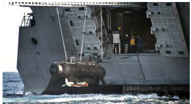
Figure 2 | The AN/AQS-20A is the only system certified for deployment from the Navy's Littoral Combat Ships. Photo courtesy of Raytheon.
